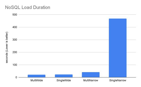
MultiWide took the least amount of time to ingest all 267,840 readings with small increases for SingleWide and MultiNarrow data models while the SingleNarrow data model took significantly longer. Calculating ingestion rates shows the differences further.
