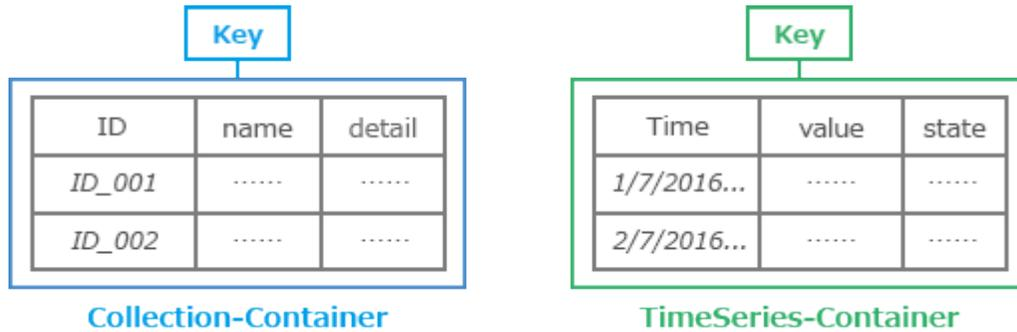
TimeSeries-Container is apt for IoT scenarios where the data is associated with a time-stamp. GridDB supports numerous time series functions such as
