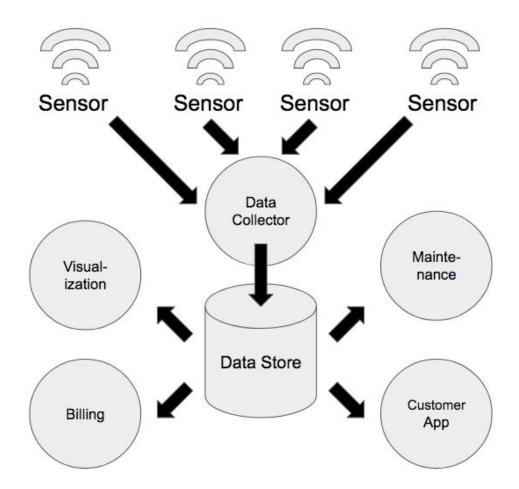
Once the data is stored in the primary data store, other processes can perform analysis or visualize the stored data either in real time or in batches.
