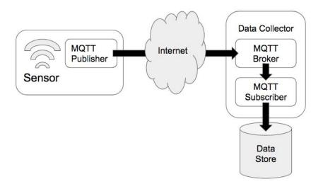
The MQTT broker is a service that runs on the data collector and passes data between the MQTT publisher that is executed within the sensor or edge device and the MQTT Subscriber that reads the publisher's data and writes it into the data store. Popular brokers include Mosquitto<sup>2</sup>, HiveMQ<sup>3</sup>, and RabbitMQ<sup>4</sup>, any of which can be used within CroMFlaG2.
