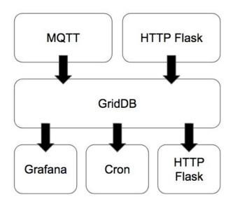
In CroMFlaG2, the MQTT Broker and Subscriber or HTTP Flask Application act as the data collector while GridDB is the data store. HTTP Flask can also operate as an endpoint to provide real time data to untrusted applications, for example, those developed or executed by third parties outside of the data hosting organization. Meanwhile Grafana provides a platform to visualize the data and Cron is used to generate reports, invoices, etc. on predefined intervals.
